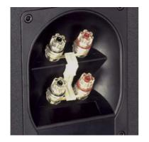
The high-quality terminals with separate circuit boards for bass/midrange and treble circuits are easy to access and allow larger cable diameters (16 mm²), as well as high-quality spade connectors (e. g. WBT products) with diameters of max. 8 mm.
