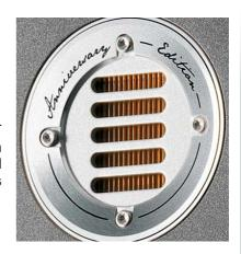
Strong drive and a new neodymium magnet system endow the JET III tweeter with incredible dynamic reserves and a high maximum output level. A new inner structure, and larger sound apertures, yield a precise upper cut-off frequency of 50 kHz. The JET III tweeter is therefore ideal for the reproduction of DVD-A, SACD and Vinyl.
